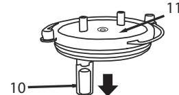
2. Remove the float (.10a) from the safety device (.10)
