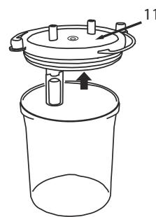
1. Remove the safety device (.10) from the canister lid (.11)
